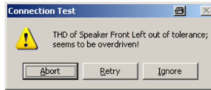
Fig. 82 Warning for excessive total harmonic distortion of a speaker.
