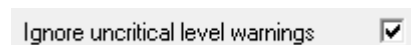
Fig. 85 Checkbox for suppressing the message caused by excessive single level deviation and other uncritical warnings.
