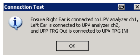
Fig. 75 Instructions for change of cabling during the calibration process.
